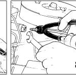
Brake Tube Pliers allows a tight 90° bend on the brake tube, right at the tube nut.
