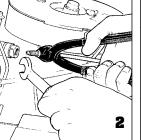
Brake Tube Pliers allow you to align the tube nut during assembly. In addition, it grips 3/16" or 1/4" brake tube securely without damaging it.
